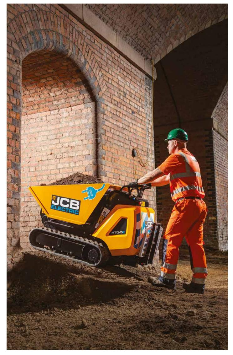
Offering walk-behind and ride-along capability, the HTD-5E makes moving material easy for the operator across multiple applications.
