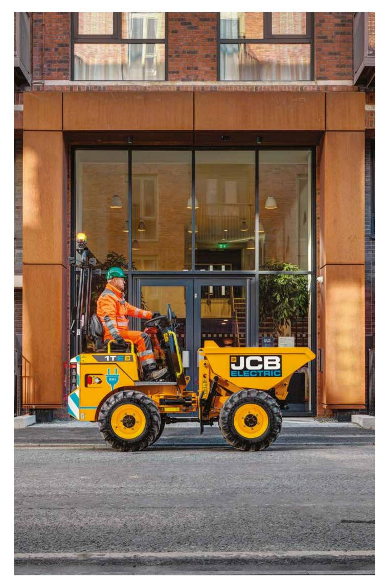
Built to withstand the toughest job sites, the High-Tip skip allows the ITE to unload material into large containers, whilst its compact design enables working in confined areas.
