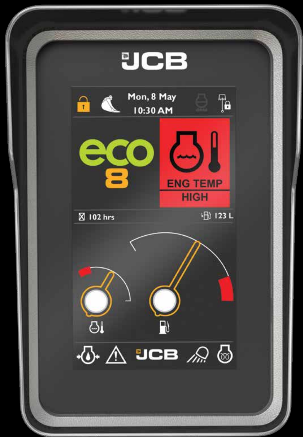
Display of all critical parameters for easy health monitoring
