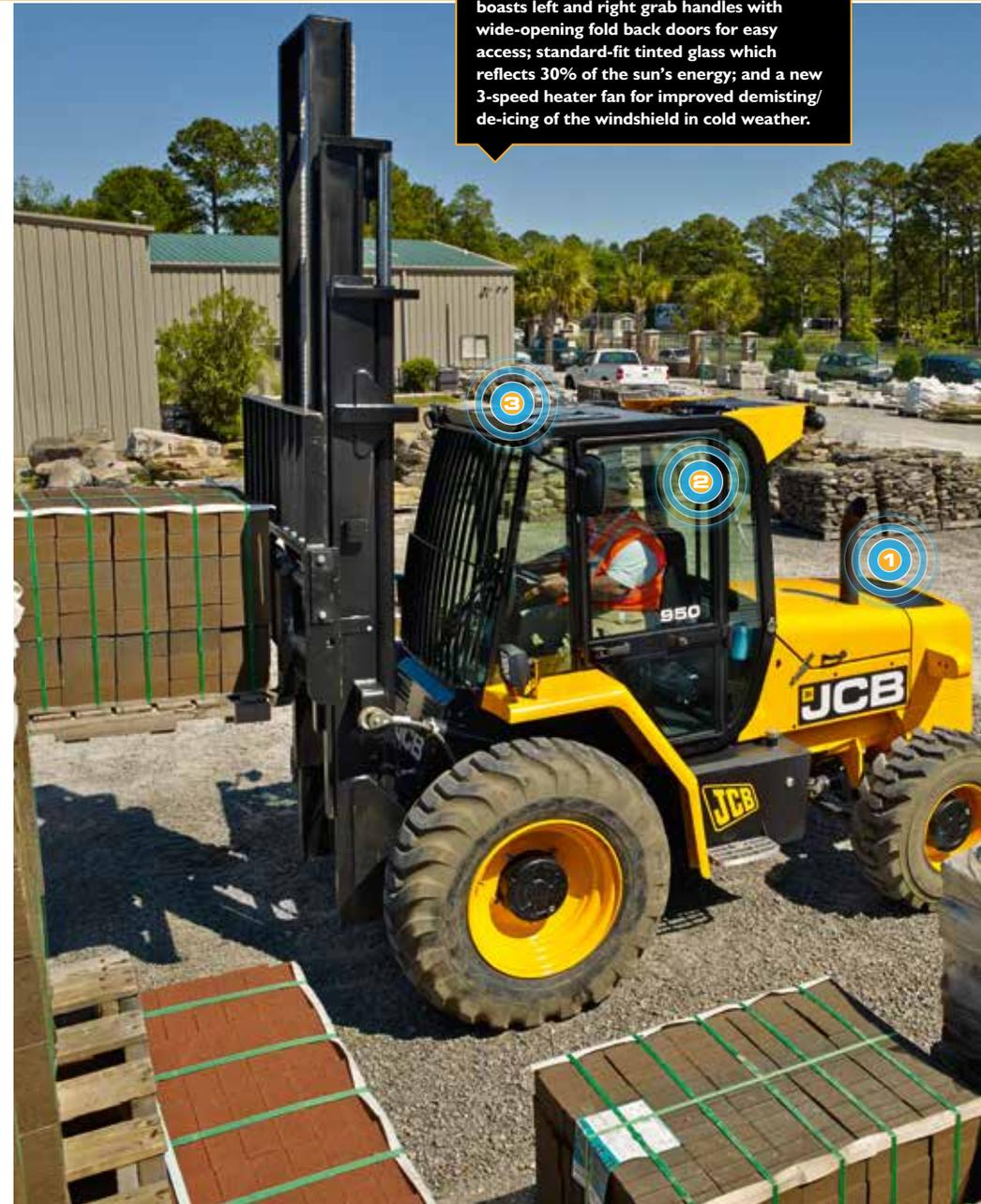
The large, spacious cab of our new RTFLs boasts left and right grab handles with wide-opening fold back doors for easy access; standard-fit tinted glass which reflects 30% of the sun's energy; and a new 3-speed heater fan for improved demisting/de-icing of the windshield in cold weather.
