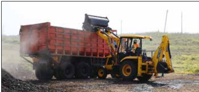
High dumper (hywa) loading
