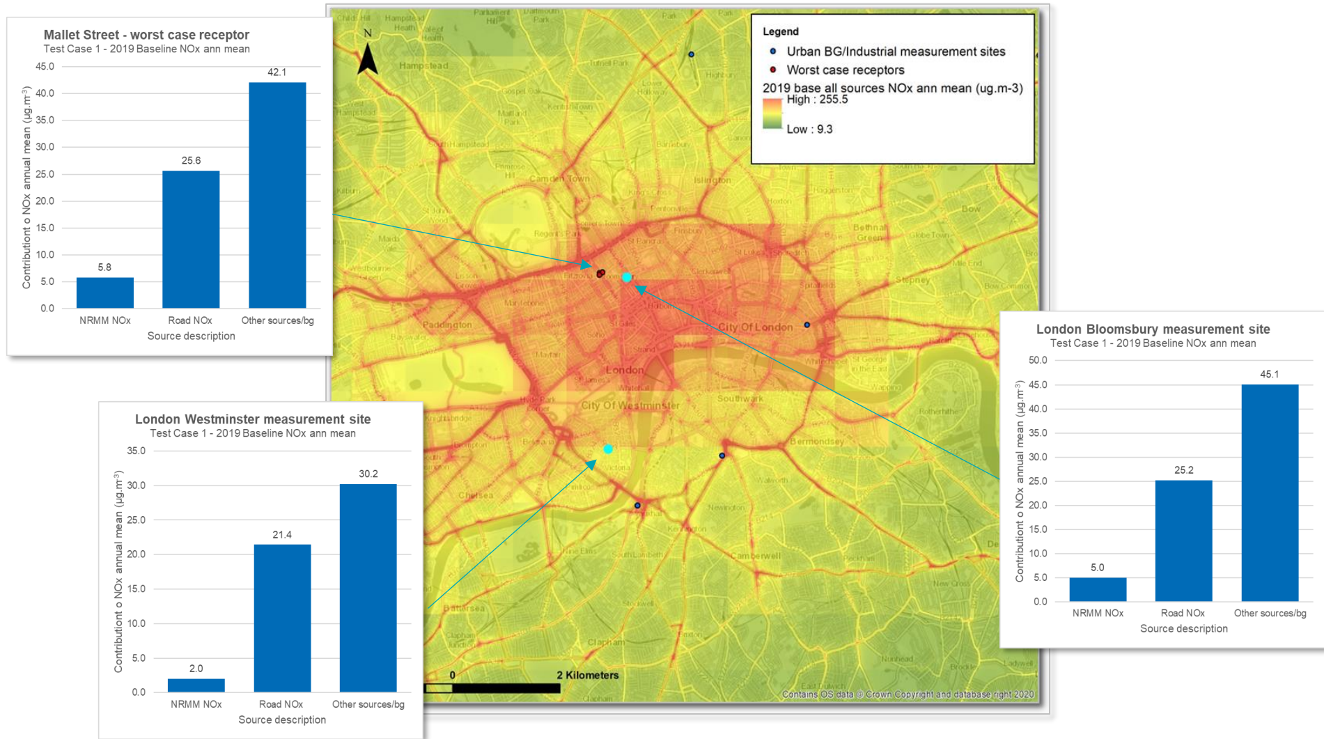
Figure 14: 2019 Baseline NOx annual mean mapped model results and source apportionment at three locations
