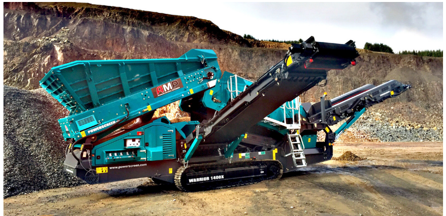
The Terex Powerscreen Warrior 1400X screener – now powered by a JCB Stage V IPU engine. ▲
