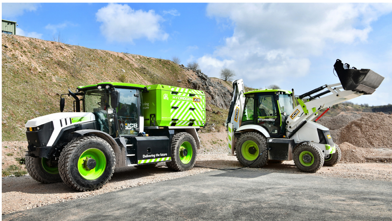
The JCB Mobile Refueller (l) with JCB's 3CX backhoe loader (r) powered by a hydrogen combustion engine. ▲
